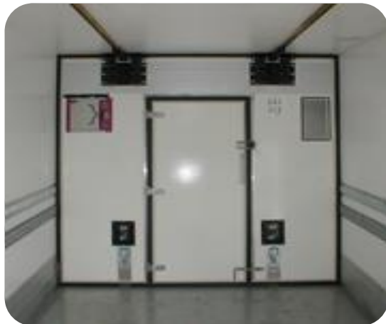
Refrigerated Box – Door inside partition wall
