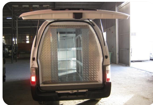
Chiller Van with rack system
