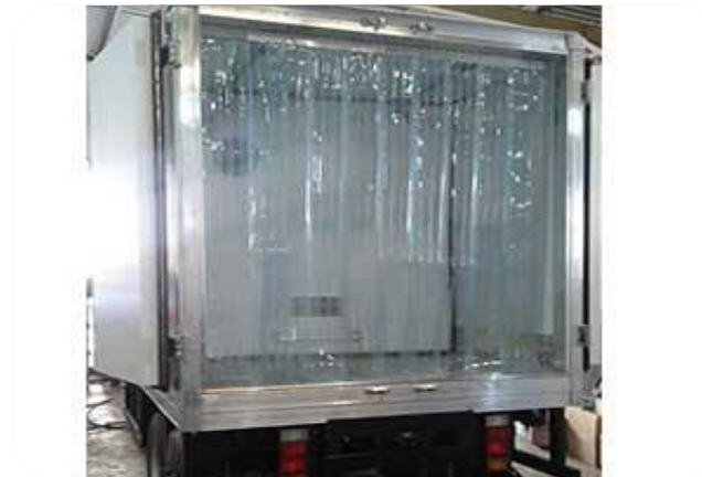
Refrigerated Box with plastic curtain
